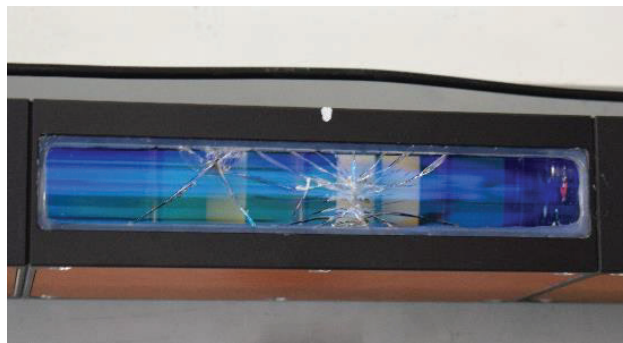
Figure 13. A cracked lens of an IR light screen due to fragment impact.
