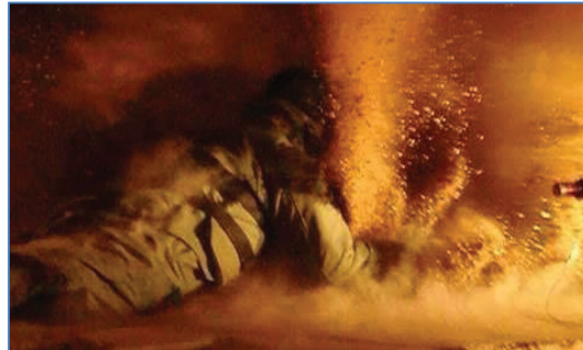
Figure 4. Secondary fragmentation from a buried anti-personnel mine (Courtesy: OTS Ltd)
