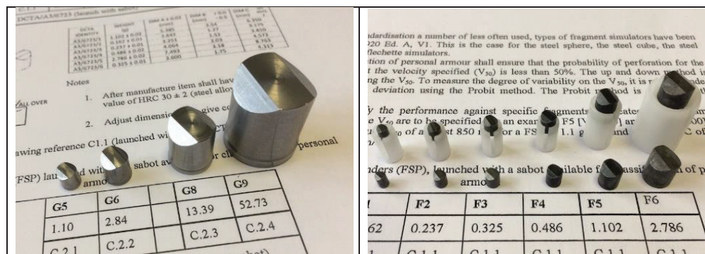
Figure 1. Pictures of fragments defined in current AEP 2920 [2] [4] - Left: “G” fragments with skirt- Right: “F” fragments without skirt
