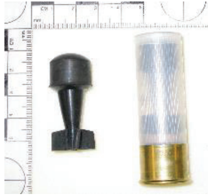
Figure 3. 12-gauge rubber round and cartridge.
