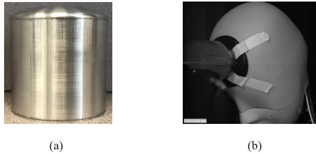
Figure 12. Aluminium projectile used in air cannon testing on front ballistic crown (a). Projectile impact on front ballistic crown (b).
