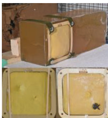
Figure 5. Skin Surrogate and Ballistic Gelatin utilized for penetration testing.
