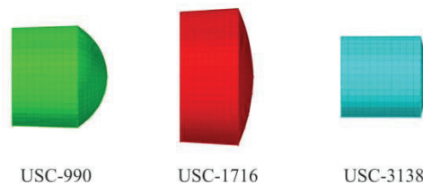
Figure 8. Equivalent projectile geometry for three field cases.
