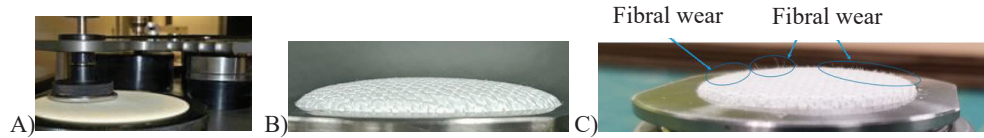
Figure 15: Martindale test ISO 12947-2 (ASTM D 4966); A) testing the abrasion resistance of the knit fabric sample; B), C) Knit specimen after abrasion > 150.000 test cycles, B) shows no wear, C) shows slight fibral wear.
