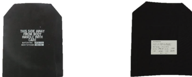
Photo No. 3 Re-built Excessively Used (Worn-out)/Aged Hard Armour Insert (2013 Production).
