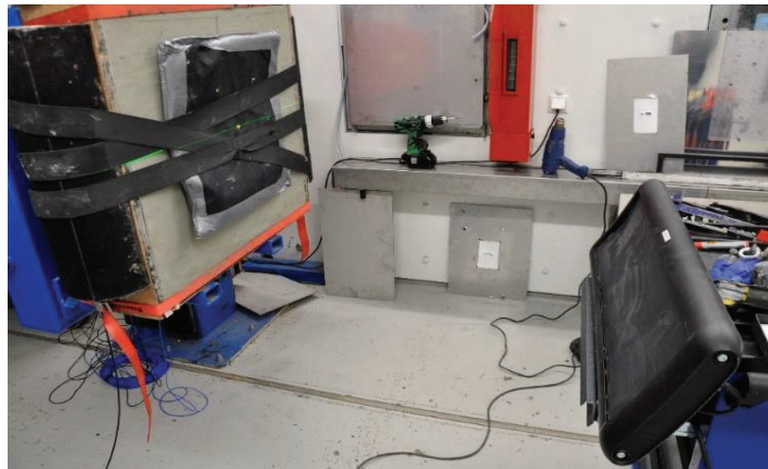
Figure 5. Infra-red heater (lower-right) in front of the instrumented clay box allowed the temperature to be constant and provided access for personnel.
