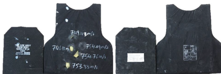
Photo No. 5 Status of Non-Used (Aged)/ Stored Inserts (2013 Production) ICW 3A 9mm Vest No Complete Penetration
