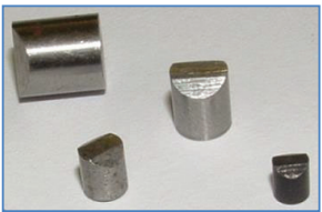
Figure 8. Typical chisel-nosed FSPs (Photo: PGC)
