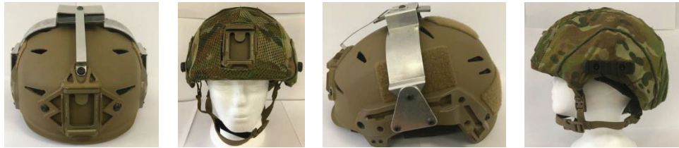
Figure 1. Trial helmets – mass adjustment rig and helmet cover
