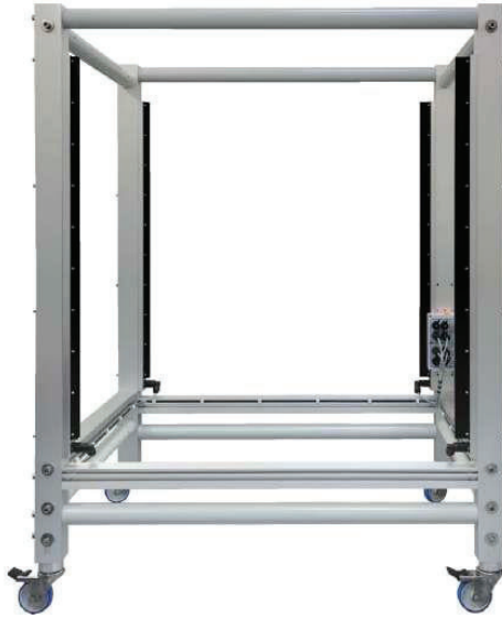
Figure 8. Example of a wheeled mobile velocity measurement instrument
