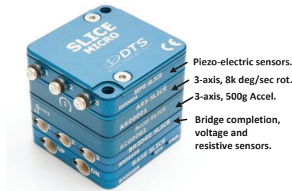
Figure 3. Reconfigurable data acquisition system.
