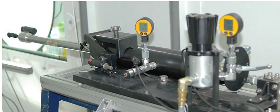
Figure 4. An example of a modern gas-gun: the UK Sabre gas gun weapon system fitted with an 800 mm barrel
