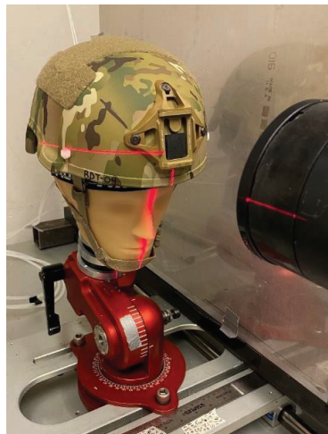
Figure 1. Photograph of the helmeted headform with the end cap of the linear impactor visible.
