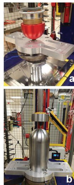
Figure 4: Impact test set-up for Phase 1 (a) and Phase 2 (b)
