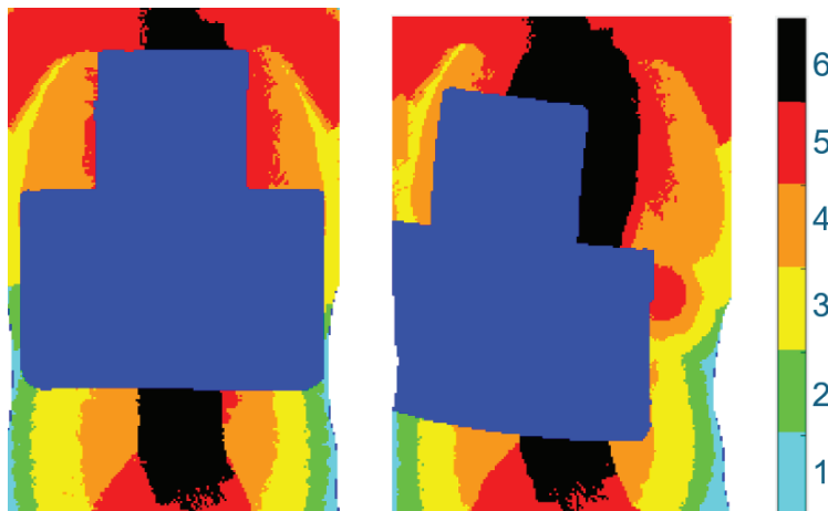
Figure 8. Example of output from WTI model. The blue area represents shotlines being stopped by the hard plates, the other colours correspond to AIS 1-6 as shown in the scale.
