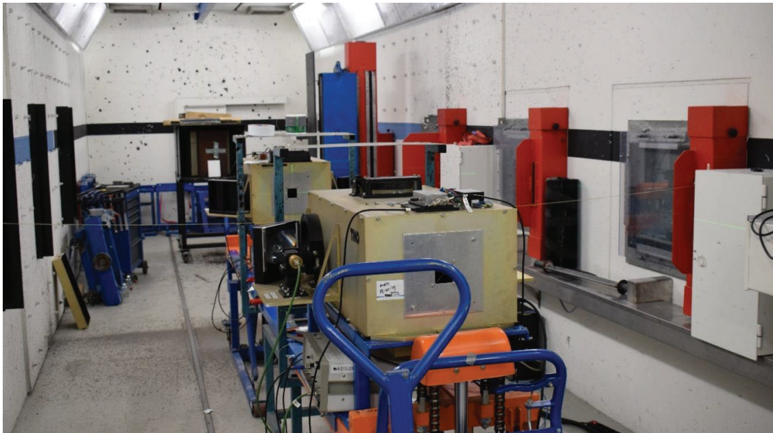
Figure 3. Overview of the setup in one of the small caliber ranges. The red boxes on the right are wall mounted IR light screens, the black boxes on the left are the reflectors. The calibration units are positioned in the line of fire and just in front of light screen 1 and behind light screen 2.
