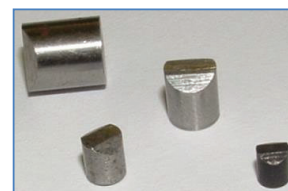
Figure 8. Typical chisel-nosed FSPs (Photo: PGC)
