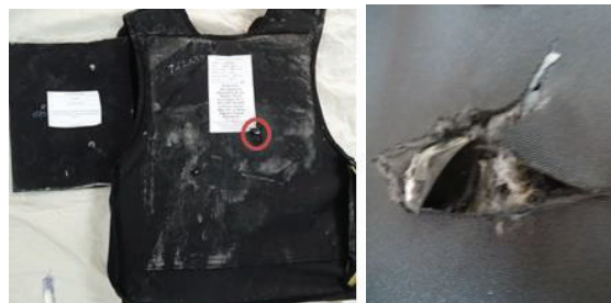
Photo No. 4 Status of Excessively Used (Worn-out)/Aged Inserts (2013 Production) ICW 3A 9mm Vest, Complete Penetration
