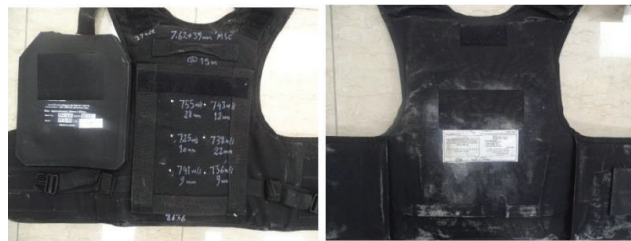
Photo No. 6 Status of Re-built Excessively Used (Worn-out)/Aged Inserts (2013 Production) ICW 3A 9mm Vest, No complete Penetration and BFS Depths are less than 44mm
