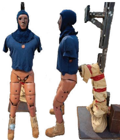
Figure 3. Surrogate system mounted to the steel blast test stand. The stand included a plate to mount the HSTM and the Hybrid III pelvis and a head support to prevent excessive torso hyperextension.
