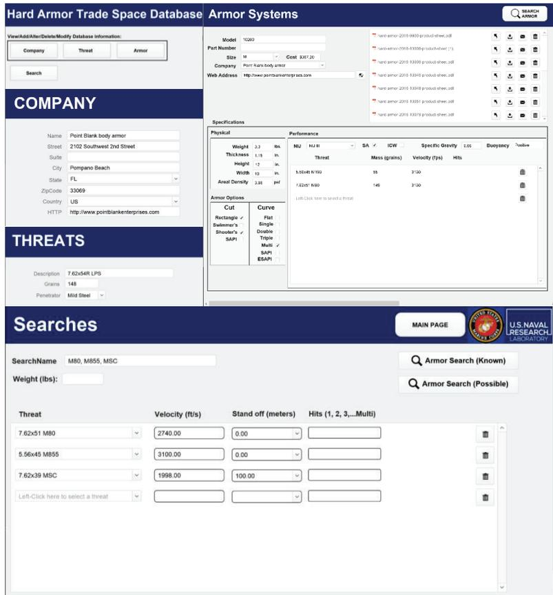
**Figure 4.** Hard Armour Trade Space analysis system comprised of a database built from a common database development system. Shown (upper left) the main page, the page for Company input, and Threat input, (upper right) Armour system input, and (lower) the search page for finding the required armour.
