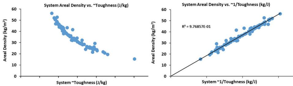
**Figure 7.** Data from Figure 6 transformed to show armour performance trend. (left) Data from the lower right plot of Figure 6 normalized by dividing the threat projected energy by the area density to produce an armour ‘toughness’ metric. (right) the same data from the plot on the left but representing the inverse ‘toughness’.
