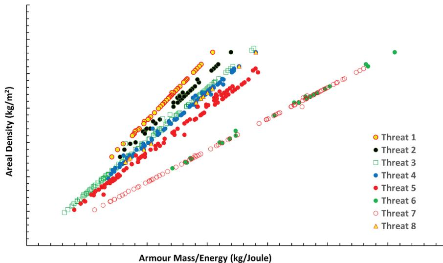
**Figure 8.** Plot of armour areal density vs the armour mass per unit energy which the armour system is known to absorb based on ballistic test reports. Each point represents a specific armour system/threat pair for which the armour was tested.
