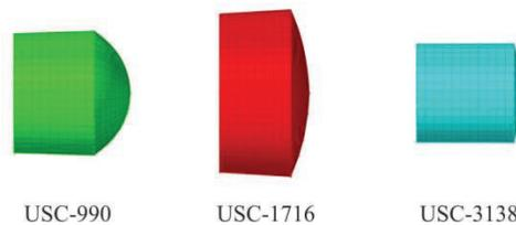
**Figure 8.** Equivalent projectile geometry for three field cases.
