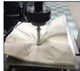
Figure 13: Dynamic flex testing, PED-IOP-008 [16].
