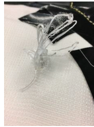
Figure 5: Yarn pull out after fragment impact.
