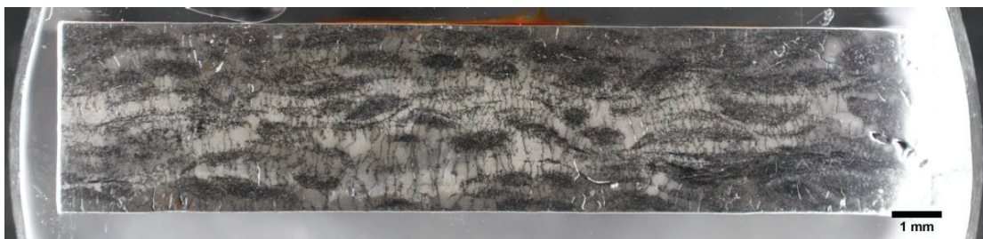
Figure 5. Optical photograph of polished cross-section that was cut parallel to the z-direction.
