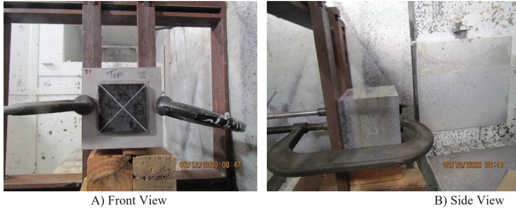
Figure 8. Test setup for SiC targets in ballistic investigation.
