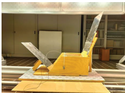
Fig. 1. Original foldable solar cooker
