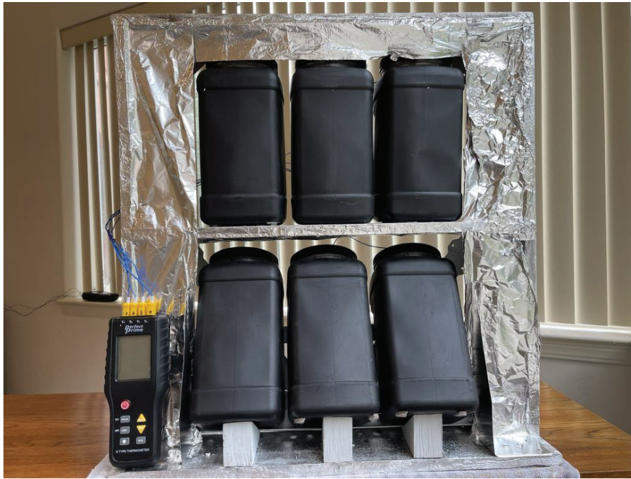
Fig. 1. Experimental setup showing six flat black painted and water-filled containers on a shelf. The containers on the lower shelf are tilted at 60° and those on the upper shelf are tilted at 90°. (Photo credit: Martin Smullen)
