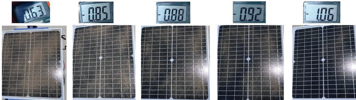
Fig. 8. Nonlinear panel output vs. applied dust amount (Photo credit: Xiuhua Si.)
