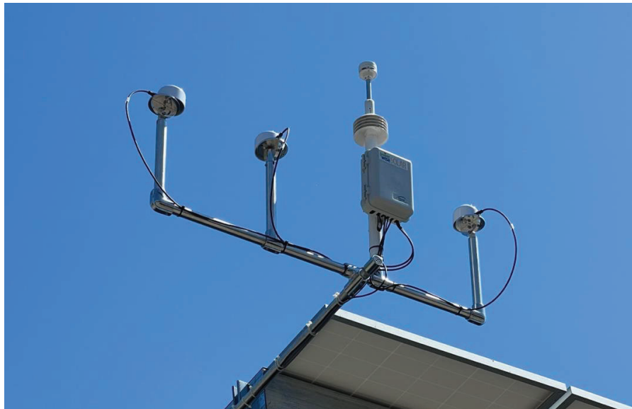
Fig. 1. Solar irradiance and weather monitoring station co-located in University of the Pacific's parking lot 4.
