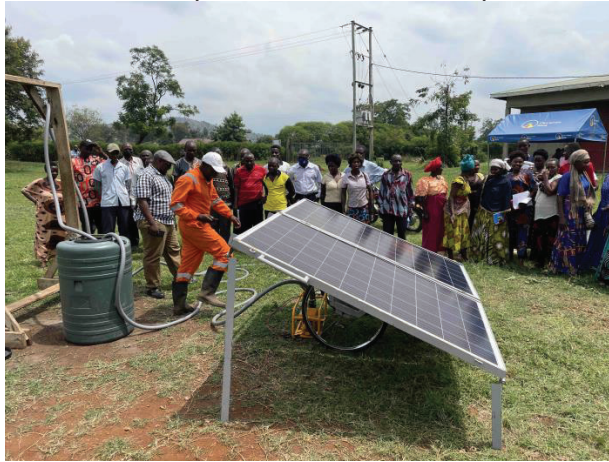
Fig. 1. The USDA farmer training by Green Powered Technology uses a portable solar water pump system with a folding array mounted on bicycle wheels for transportation. It was for crop irrigation that was shared between several farmers at the Rugendabara Coop in western Uganda in August 2022. It uses the world's only surface helical rotor pump, developed by Ennos. (Credit: Robert Foster)
