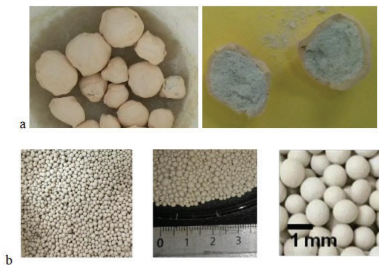
Figure 3. Green nearly spherical formulations: a. Core-shell pellets (clay coated Ca(OH) 2 cores), b. CaO/clay composite pellets
