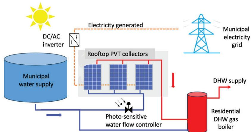
**Figure 1:** A schematic of the physical model of the proposed configuration.
