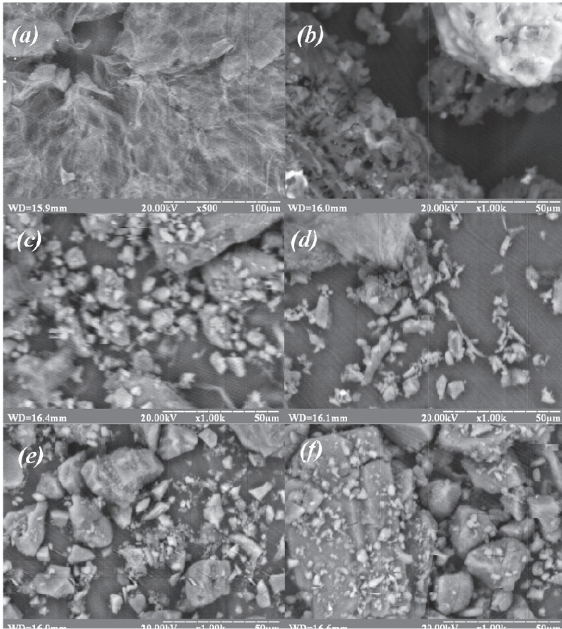
**Figure 2:** SEM images of: TEG (a); CNT (b); As-TEG biocomposite (c); GI-TEG biocomposite (d); As-CNTs biocomposite (e); GI-CNTs biocomposite (f).
