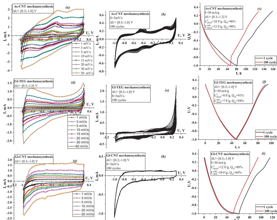
**Figure 4:** CVA curves of electrochemical systems based on As-CNT, GI-TEG, GI-CNT bio-composites in the range [0.3 to -1.0]V (a, d, g), CVA profiles at the 3mV/s during 100 cycles for As-CNT (b), GI-TEG (e), GI-CNT (h) bio-composites; 1<sup>st</sup> and 100<sup>nd</sup> charge/discharge galvanostatic cycles at the current 30mA/g in the range [0.3 to -1.0]V for As-CNT (c), GI-TEG (f), GI-CNT (i) bio-composites.
