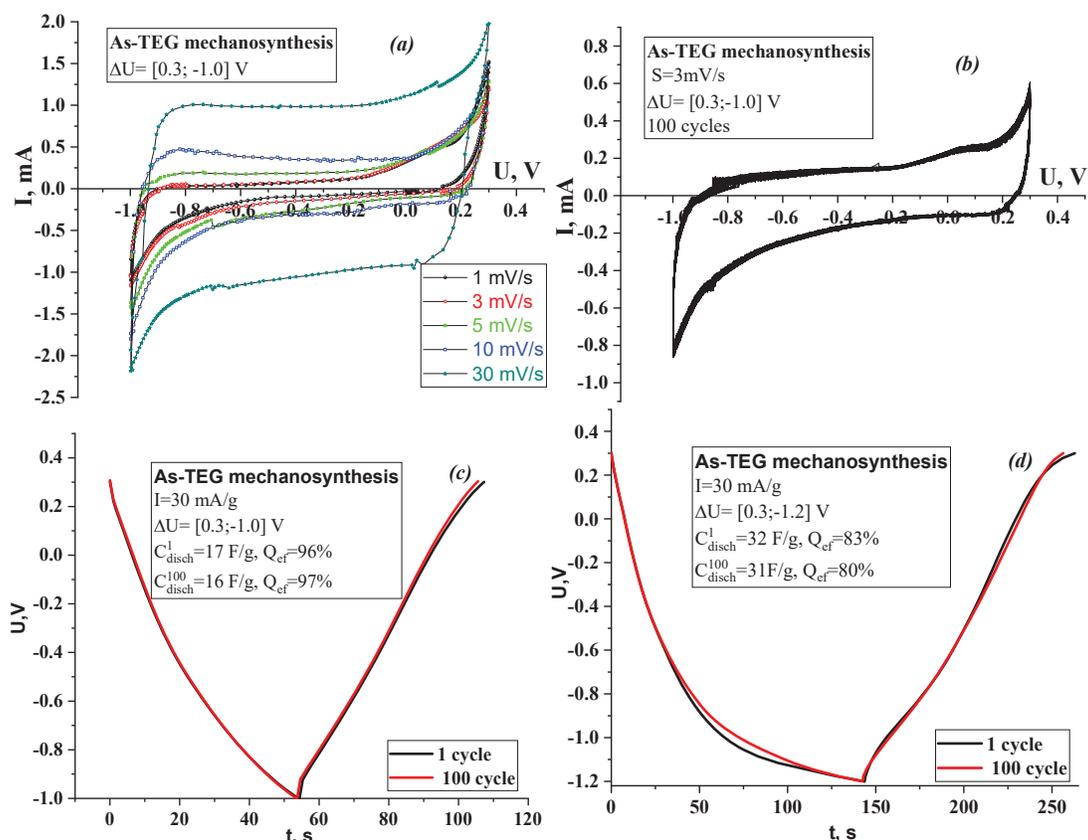
**Figure 3.** CVA curves of electrochemical systems based on As-TEG bio-composite in the voltage scanning range of 0.3 to -1.0V (a); CVA profiles at the 3mV/s during 100 cycles (b); 1<sup>st</sup> and 100<sup>nd</sup> charge/discharge galvanostatic cycles at the current 30mA/g in the range of 0.3 to -1.0V (c) and 0.3 to -1.2V (d).
