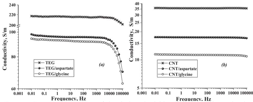
**Figure 1:** Frequency dependence of electrical conductivities of bio-composites and carbon templates
