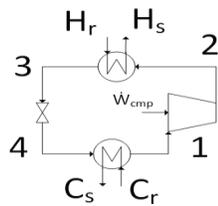
**Figure 1:** The physical structure of the heat pump system
