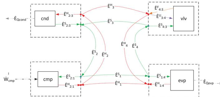
Figure 6: Physical-Productive Diagram of the heat pump system using the H&S Model with Localized UFS Model
