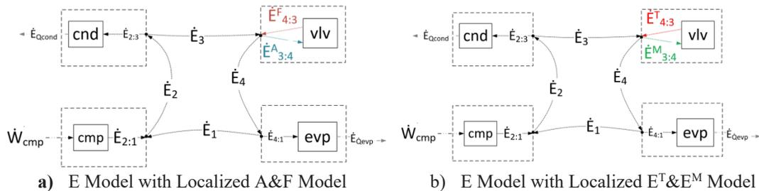
**Figure 3:** Physical-Productive Diagram of the heat pump system
