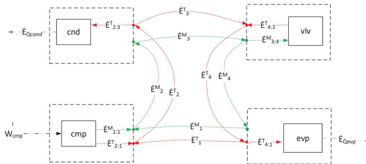
**Figure 4:** Physical-Productive Diagram of the heat pump system using the E<sup>T</sup>&E<sup>M</sup> Model
