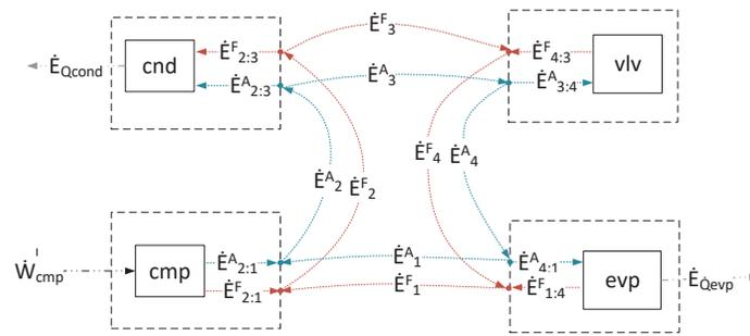
Figure 5: Physical-Productive Diagram of the heat pump system using the A&F Model
