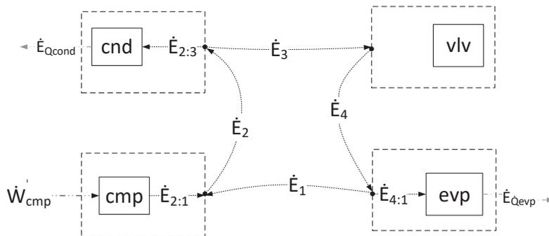
**Figure 2:** Physical-Productive Diagram of the heat pump system using the E Model
