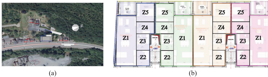
Figure 2: Building assessed a) location in Belgium, b) zone discretization for the 1 st and 2 nd floors
