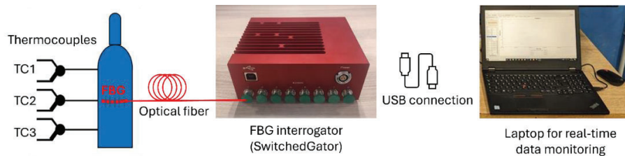
Figure 7: FBG sensor setup and data acquisition system.
