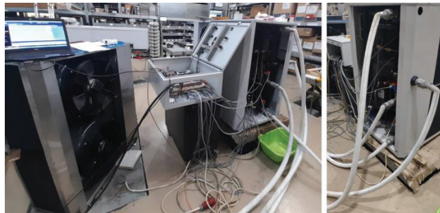
Figure 2: Lab tests of the heat pump unit (right), and the connections with cold and hot water (left).
