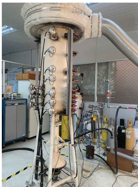
Figure 2: Vertical combustion chamber.
