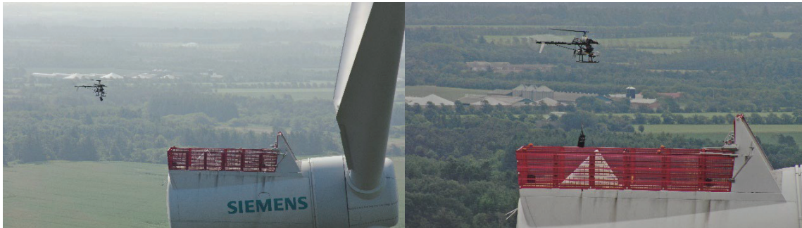
Figure 13. Approach and payload delivery with the Scout B1-100 UAV helicopter (courtesy Aalborg University, Drone Research Lab)
