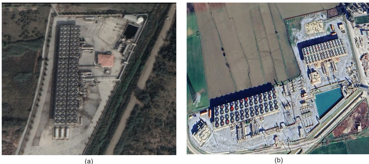
Figure 8. ORC plants of up to 50 MW with geothermal heat sources: a) one of 22.5 MW, of two (Ken Kipaş), b) two of 24 MW (Kubilay I, II)
