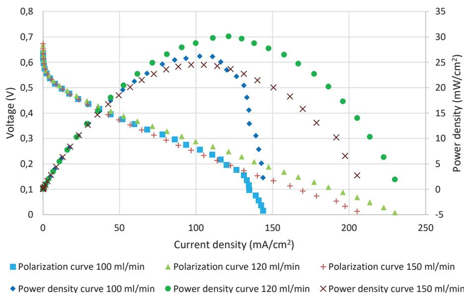
**Figure 3.** Polarization and power density curves of the DMFC single cell for different oxygen flow rates obtained at a temperature of 60 °C, pressure of 1 bar and a methanol concentration of 1 M and flow rate of 3 ml/min.
