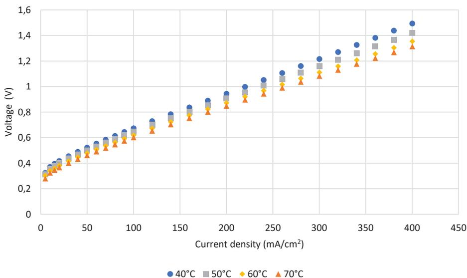
**Figure 4.** Polarization curves of the methanol electrolyser single cell for temperatures of 40 °C, 50 °C, 60 °C and 70 °C obtained with aqueous methanol of concentration 1 M and methanol flow rate of 6 ml/min.
