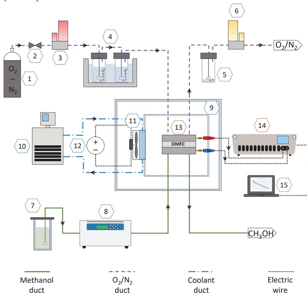
**Figure 1.** Diagram of the test bench when it is used to test Direct Methanol Fuel Cells. 1 - Compressed O<sub>2</sub>/N<sub>2</sub> cylinder. 2 - Pressure reduction valve. 3 - Gas flow controller. 4 - Gas humidification system. 5 - Water trap. 6 - Gas pressure controller. 7 - Aqueous methanol tank. 8 - Methanol pump. 9 - Chamber. 10 - Refrigerated and heating circulator. 11 - Heat exchanger. 12 - Power source. 13 - DMFC. 14 - Potentiostat-galvanostat. 15 - Computer.
