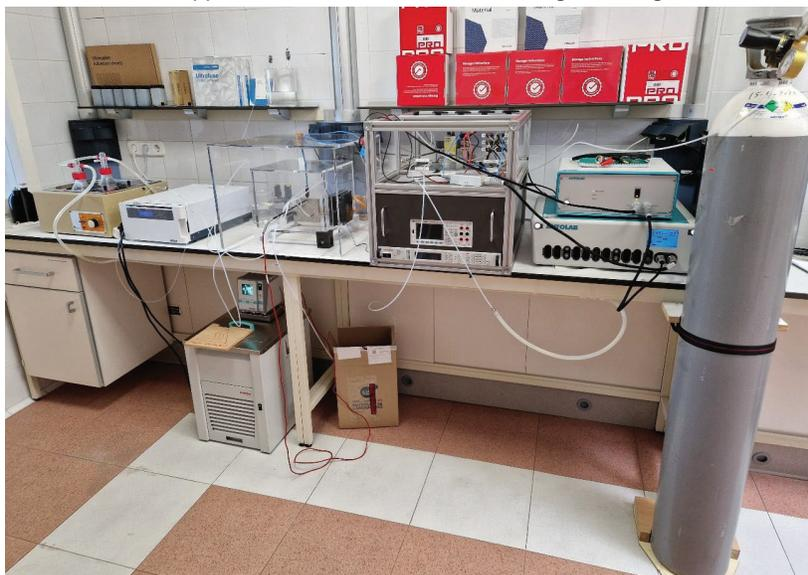
**Figure 2.** The test bench designed and built to study DMFC and methanol electrolysers.
