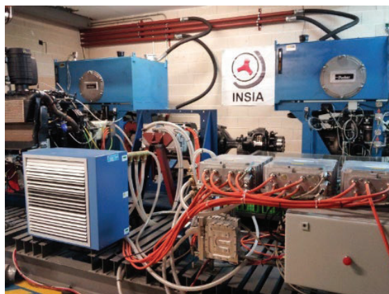
Figure 6: Test bench for hybrid power trains.
