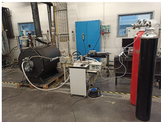
Figure 8: Combustion chamber CO 2 lung (combustion tests of the ternary mixture CH 4 /CO 2 /H 2 ).
