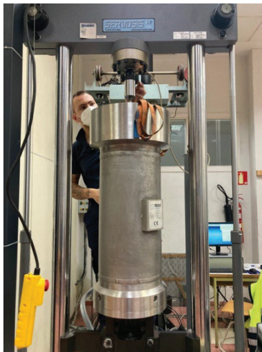
Figure 5: High pressure hydrogen chamber for material testing.
