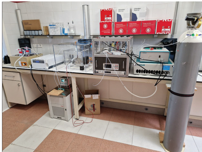
Figure 2: Test bench for direct methanol fuel cell and methanol electrolyser
