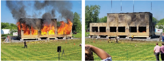
Figure 22: Ottawa Mass Timber Fire Demonstration Test during and after the test as the fire died down
