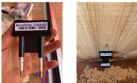
Figure 9: A MC sensor with heat-shrink tubing and 20 mm exposed screw tip (left), then embedded in to the CLT wall (right) in the residential CLT building in Cairns
