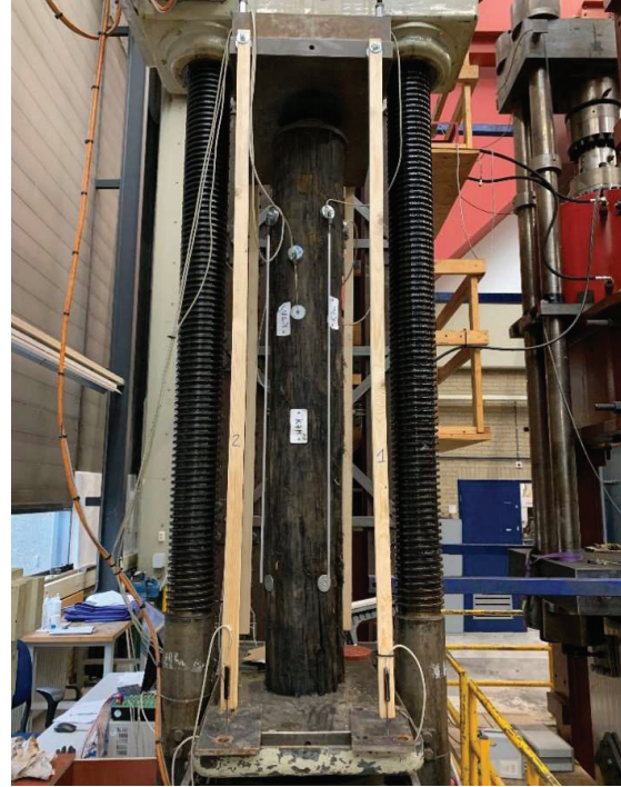
Figure 2: Setup for compression tests.
