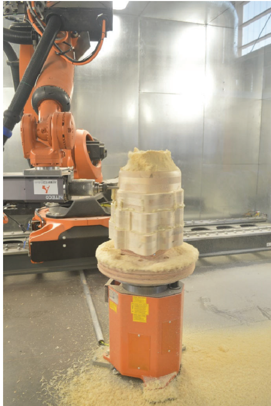
Figure 6: KUKA robotic arm milling Squall prototype
