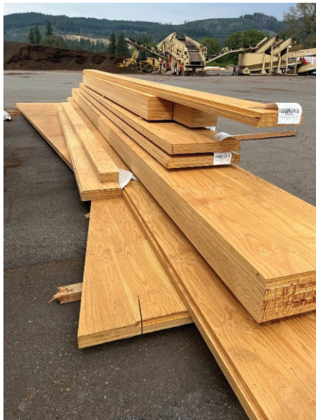
Figure 2: MPP saved scraps, of a scale and dimension suitable to furniture reuse but irregular and impractical for building applications.
