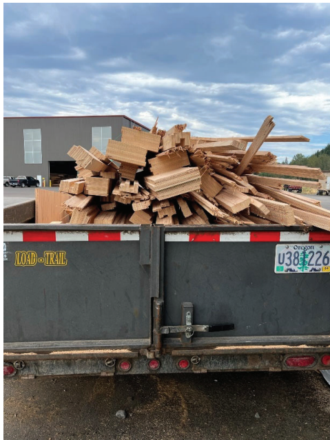
Figure 1: Thinner and small scale scraps of MPP suitable for chipping and cogen collected at Freres' Cedar Mill facility.
