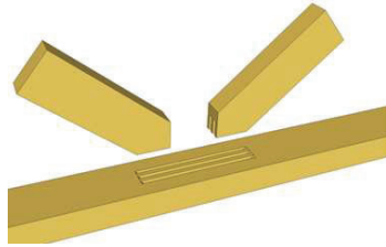
Figure 1: DSB joint, the fingers are not tapering and the webs are not connected to each other.
