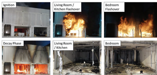
Figure 3: Fire Test 1 test progression photos
