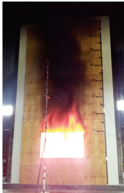
Figure 7: Example CAN/ULC-S134 test
