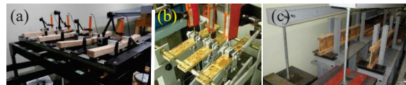
Photo 1: Tests to evaluate the duration of load for (a) the flange of LVL, (b) the web of OSB and (c) I-joint.
