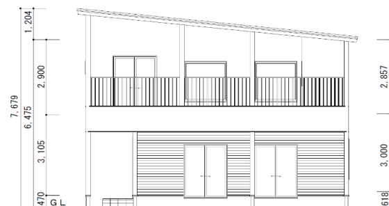
Figure 2: South elevation of the prototype house
