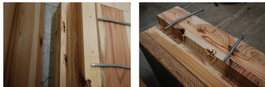
(a) Major axis specimen (b) Minor axis specimen Figure 16: Specimen after shear loading test
