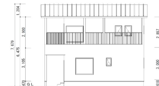
Figure 3: East elevation of the prototype house
