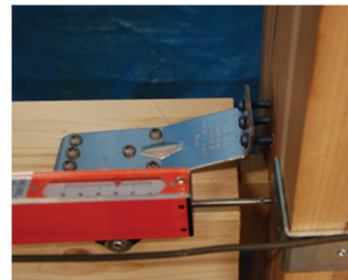
Figure 24: Joint of specimen after tensile loading test
