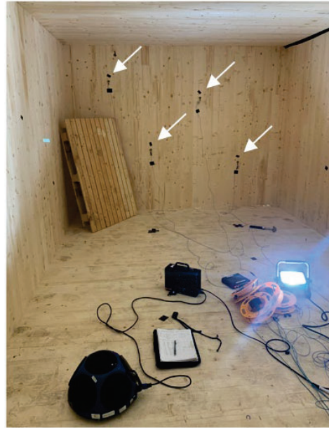
Figure 3: Photo of sensor setup inside of the test rooms. Sensor positions indicated with white arrows.
