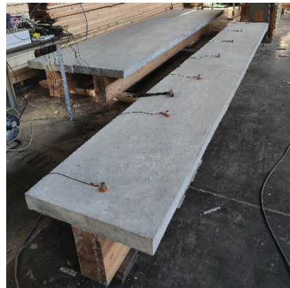
Figure 5: Dynamic test for timber-LWAC composite beam
