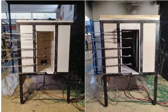
Figure 1. Indicative photos of the test compartment with inert (left) and CLT (right) ceiling installed.
