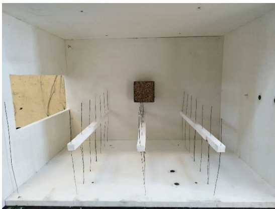
Figure 2. Indicative photo (top view) of the burner and the installed sensor network inside the compartment.
