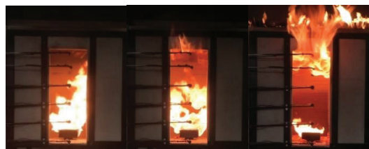
Figure 11: Photos of the “exposed CLT ceiling” fire test, 600 s (left), 1800 s (middle) and 3300 s (right) after ignition.
