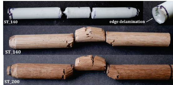
Figure 9: Failed samples, from top to bottom: GFRP in steady state at 140 °C, oak in steady state at 140 °C, oak in steady state at 200 °C.
