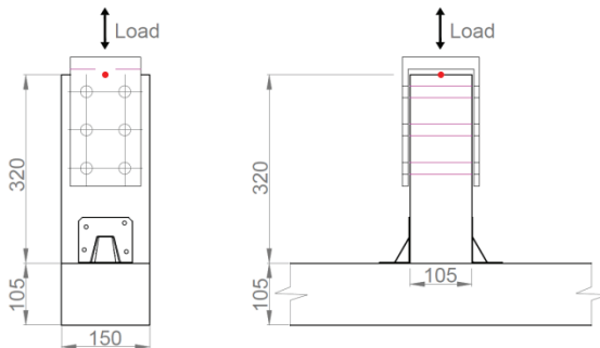
Figure 6: Front and side view of the experimental setup HGA10KT brackets for pull-out test.
