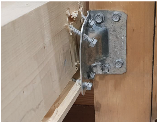
Figure 18: Test specimen with HGA10kt angle bracket and screws after shear test
