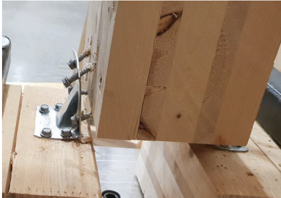
Figure 17: Test specimen with HGA10kt angle bracket and screws after pull-out test.
