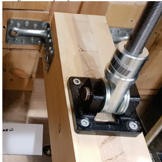
Figure 1: Experimental setup of CLT connection made of ABR9020 bracket and SDS screws subjected to rocking.
