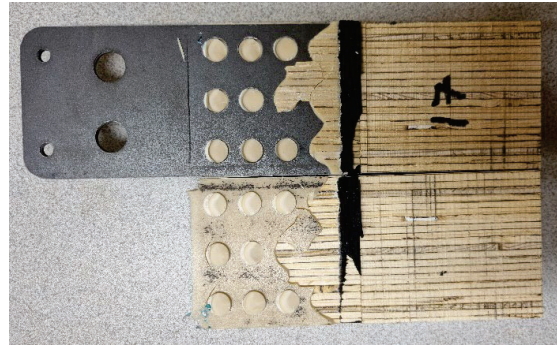
Figure 10: Combined failure in the glue dowels, the steel-to-glue interface and in the wood-to-glue interface.
