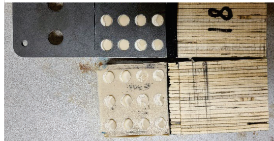
Figure 11: Failure solely in the glue dowels and in the steel-to-wood interface.
