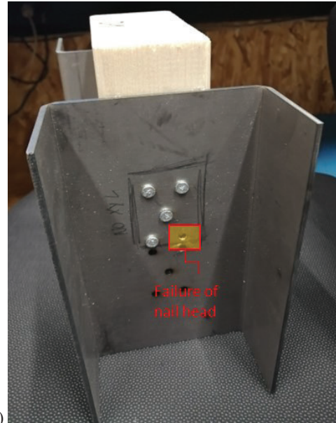
Figure 6: Samples GL-X35_02 at the end of test: a) local crushing of the timber along the grain direction and b) failure of the head of nails.
