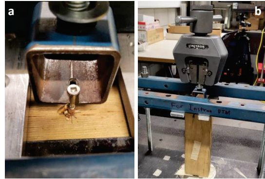
Figure 3: Screw withdrawal test setup, showing (a) grip and (b) test rig.
