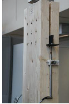
Figure 7: Small scale test setup and instrumentation.
