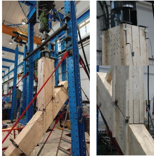
Figure 8: Diagonal test setup with three dowel connections
