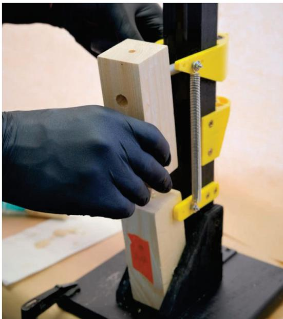
**Figure 2:** Bonding device designed for the rapid application of adhesives
