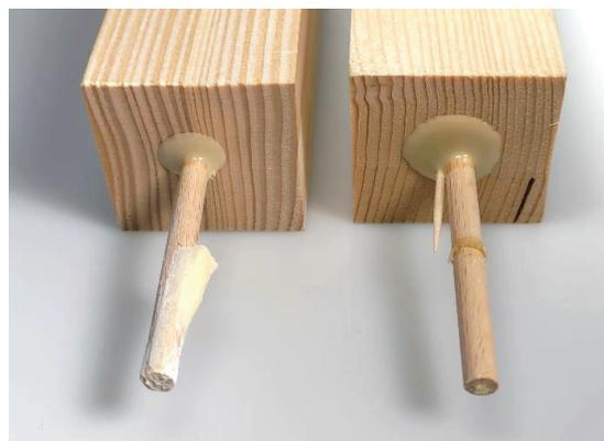
**Figure 8: Wood tear out (left) and adhesive failure (right)**
