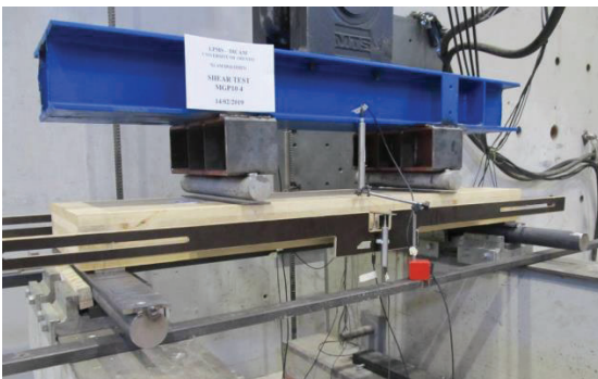
Figure 2 – The 4-point bending tests setup.
