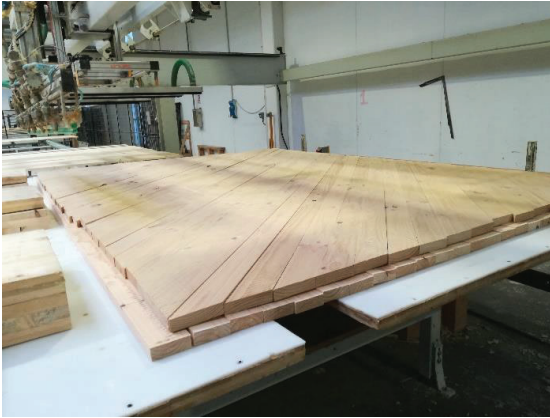
Figure 1 – The U-B45 panels (diagonal crossbands).
