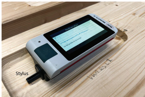
Figure 7: MarSurf PS 10 device collecting surface roughness data on bottom area of a specimen of Series B. The stylus is located below the bottom left black tube.
